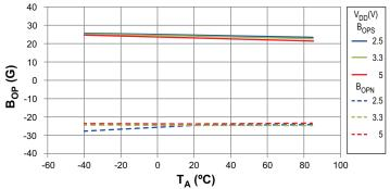
Average X-Axis Operate Point vs. Ambient Temperature
