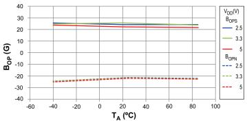
Average Z-Axis Operate Point vs. Ambient Temperature
