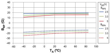
Average Y-Axis Release Point vs. Ambient Temperature
