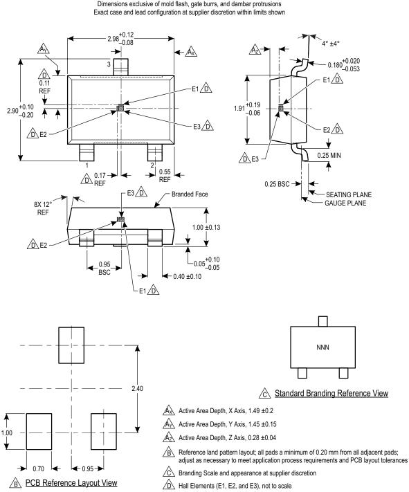
For Reference Only – Not for Tooling Use (Reference DWG-2840) Dimensions in millimeters – NOT TO SCALE Dimensions exclusive of mold flash, gate burrs, and dambar protrusions Exact case and lead configuration at supplier discretion within limits shown
