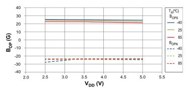
Average X-Axis Operate Point vs. Supply Voltage
