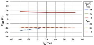
Average X-Axis Release Point vs. Ambient Temperature
