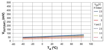
Average Low Output Voltage vs. Ambient Temperature
