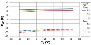
Average Y-Axis Operate Point vs. Ambient Temperature
