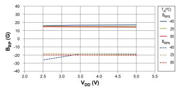
Average X-Axis Release Point vs. Supply Voltage
