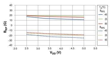
Average Y-Axis Release Point vs. Supply Voltage
