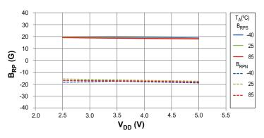
Average Z-Axis Release Point vs. Supply Voltage
