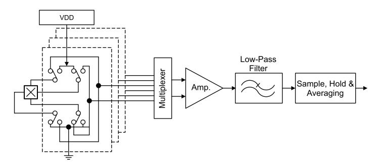
Figure 6: Model of Chopper-Stabilization Circuit (Dynamic Offset Cancellation)
