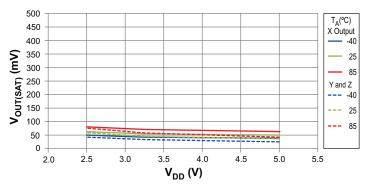
Average Low Output Voltage vs. Supply Voltage
