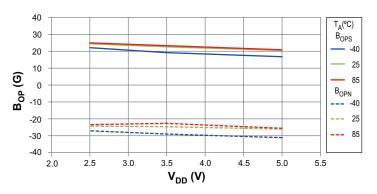
Average Y-Axis Operate Point vs. Supply Voltage
