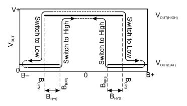
Figure 3: Switching Behavior of Omnipolar Switches
