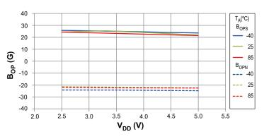
Average Z-Axis Operate Point vs. Supply Voltage
