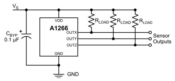
Figure 5: Typical Application Circuit for the Triple Output Selection
