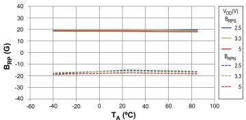
Average Z-Axis Release Point vs. Ambient Temperature
