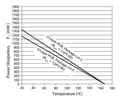
Maximum Power Dissipation versus Ambient Temperature
